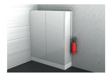
The CPS 1230 extinguishing system consists of the extinguishing nozzles with the associated supply lines, the extinguishing tank as well as the fire detection and extinguishing control system. One system protects up to two cabinets with electronic and electric components.
