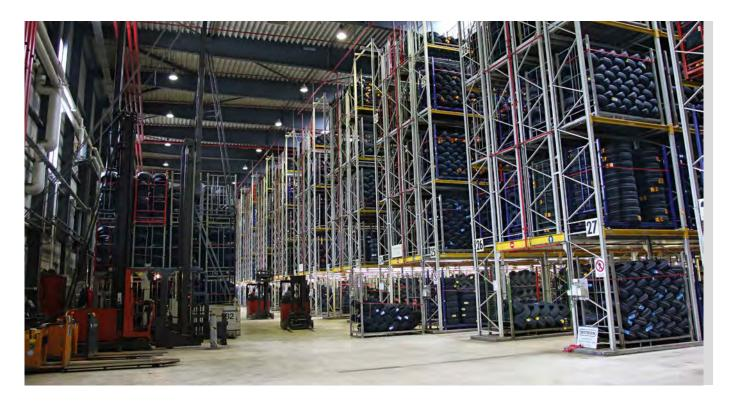
As a rule, tires are stored in block storage facilities. However, sometimes they are stored in transport pallets designed specifically for the storage of tires.
